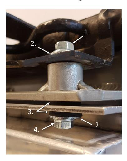
When do88 aluminum radiator is installed together with aluminum intercooler the supplied screw, two washers, two rubber washers and lock nut have to be used according to this picture.
