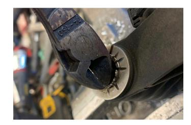
When all the strips are folded up, the steel washer and the plastic bushings can be removed.
