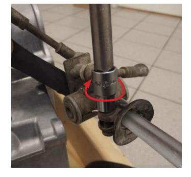
Remove the locking pins and reassemble the gaiter on the gear lever and the plastic plug in the gearbox.
