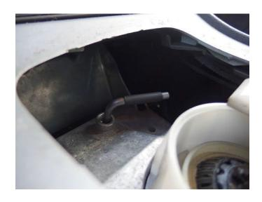
Now tighten the clamping socket on the linkage. Torque: about 25Nm.
