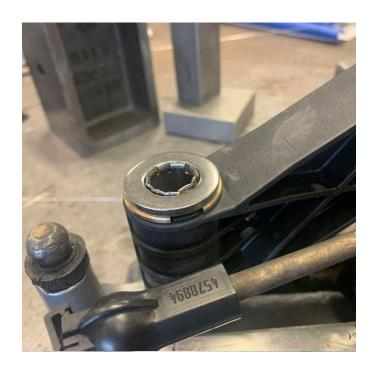
Next fasten the washer with tack welds like pictured here.
