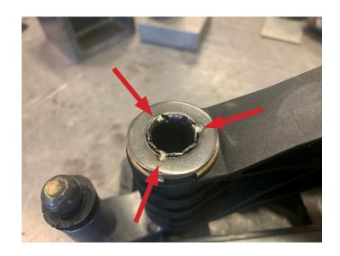
Weld all the way round the new bushing. Remember to weld a small portion and cool (e.g. with compressed air) then repeat and continue doing so until you're done. This is because the bushing is in the plastic that can easily melt from the heat that arises during welding.
